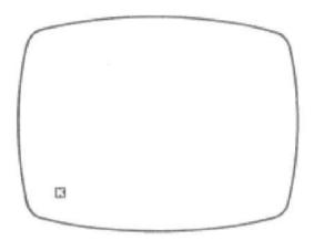
The [3] in the lower left-hand corner of the screen is called the cursor, and means the T/S 1000 is ready for action.
