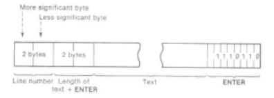
Note that, in contrast with all other cases of two-byte numbers in the Z80, the line number here (and also in a FOR-NEXT control variable) is stored with its more significant byte first: that is to say, in the order that you would write them down.
