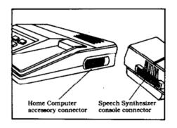
Make sure the console and the Speech Synthesizer are parallel, with the connectors aligned. Then hold the console firmly with your left hand, and gently push the Speech Synthesizer connector onto the console connector. (Note that as you face the front of the console, the product name appears on the top of the Speech Synthesizer case).
