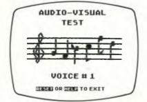
If a voice number appears but you don't hear music, that voice is not working properly. Make sure that the volume on your television is turned up. If you are using a monitor, make sure the audio cable on the monitor is firmly attached.
