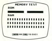
During the RAM test, 48 kilobytes(K) of RAM are tested. Each of the 48 small squares represents one K of RAM. If a square turns white, then green, the corresponding section is good. If a square turns red, the RAM section is not working.
