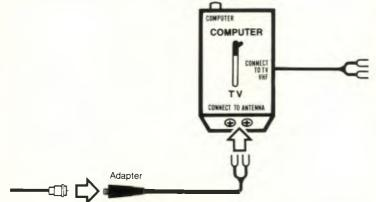
If the antenna cable is a flat twin-lead 300-OHM cable, attach it to the screw terminals on the bottom of the TV Switch Box.
