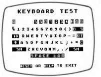
Look at the keys on the top row of the test screen keyboard. Each key except the 4 numbered keys represents a key on your keyboard. Reading from left to right, the keys in the top row include <u>Reset</u>, <u>Start</u>, <u>Select</u>, <u>Option</u>, four numbered keys, <u>Help</u>, Inverse Video, and <u>Break</u>.
