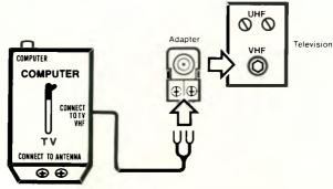
If your television has two VHF screw terminals, attach the twin-lead cable labeled Connect to TV VHF at the side of the Switch Box directly to the VHF terminals on your television.
