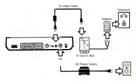
5. With the power switch on the computer in the off position, insert the round plug of the AC adapter into the Power jack on your computer. Plug the other end into an electrical outlet.
