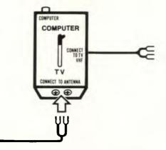
2. If your television has a threaded VHF connection, attach a threaded VHF adapter to the twin-lead cable labeled Connect to TV VHF at the side of the Switch Box and attach it to your television. (The adapter should be supplied with your television; if not, you can buy one at a video or television store.)
