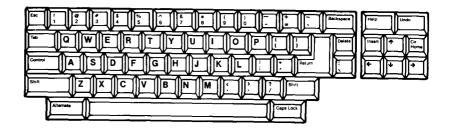
The number and symbol keys have two different characters on the key tops. Pressing either a number or symbol key produces the lower character on the key. When [Shift] is pressed, the upper character appears.
